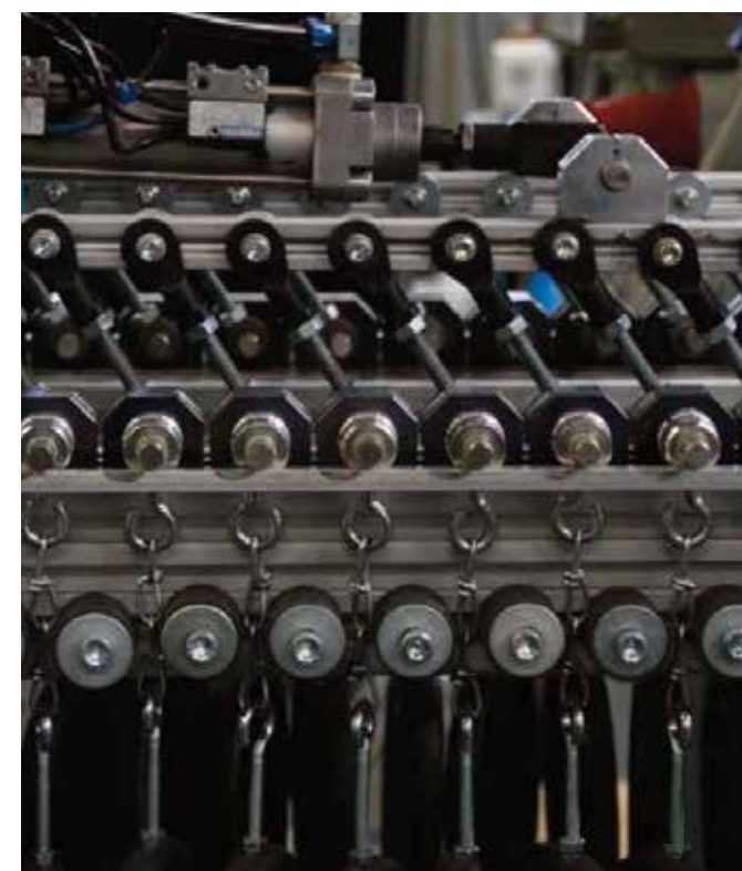
Picture 10: Pivoting wear test rig for testing the wear in pivoting movements at low loads
