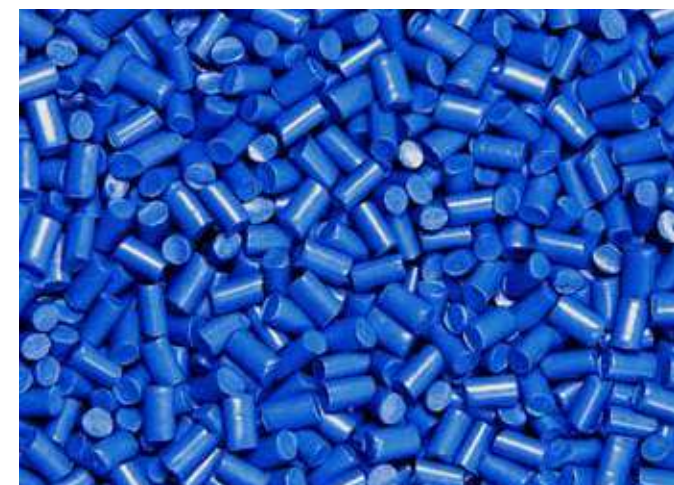
Picture 04: Polymer granulate; basis compound of the lubrication-free and predictable iglidur® plain bearings
