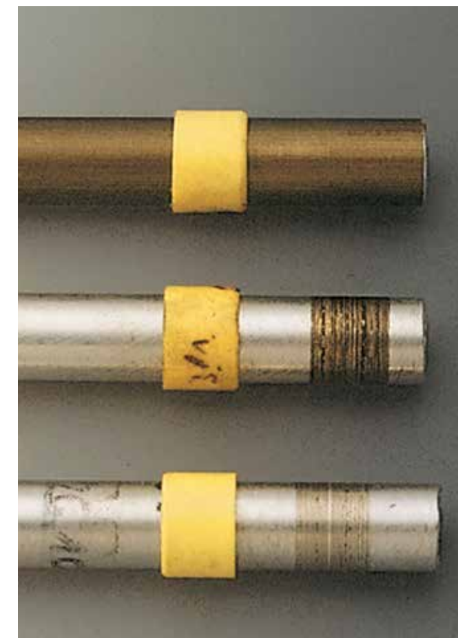
Picture 8: Wear experiments with aluminium shafts
