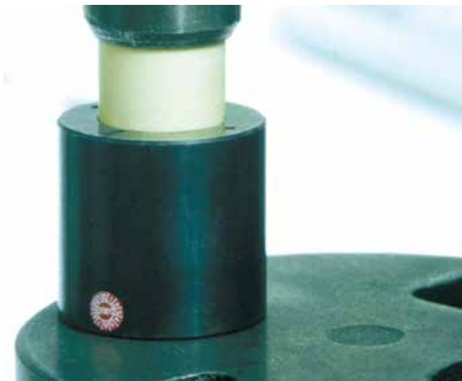
Picture 12: The bearing should be press-fitted using a flat press
