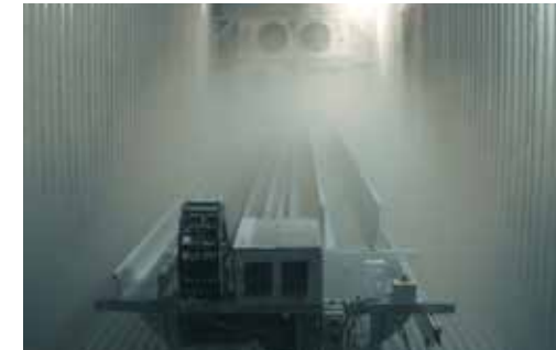
Cold tests in climatic test cabinets as low as -40°C
