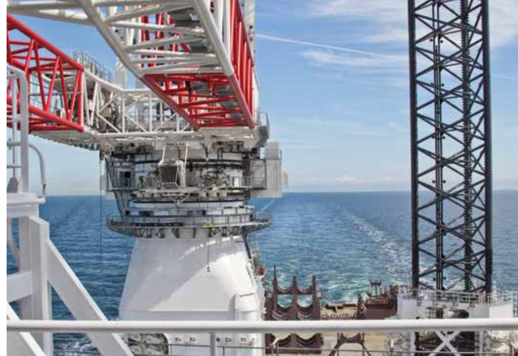
Ship crane for setting up offshore wind farms. igus® e-chains® and chainflex® cables supply power for the rotary movement of the crane.
