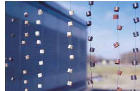
iglidur® bearing in long-term UV test
