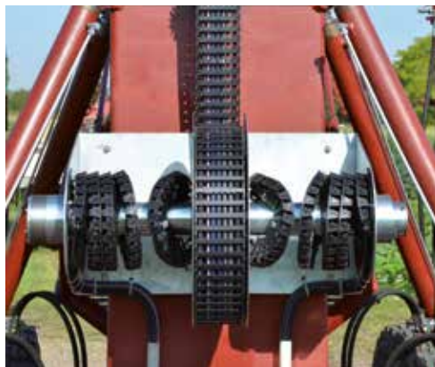
The alternative to cable reel - igus® e-spool in an extendable mast turbine system
