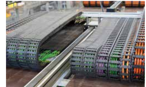
Service life experiments for e-chains® and chainflex® cables
