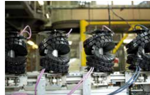
Test for torsion with e-chains® and chainflex® cables
